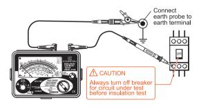
4 Check the circuit under test is not energized as follows.
