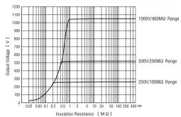
Principle of Insulation Resistance Measurement Resistance value can be obtained by applying a Certain high voltage to the resistance (insulation resistance) and measuring the flowing current.
